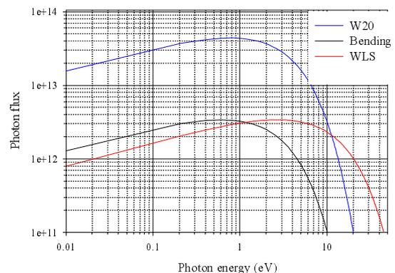
Figure 1. The comparison of spectrum of the bending magnet, wiggler and 6-T wavelength shifter (SWS).
