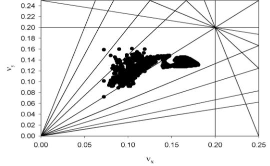
Figure 3: The tune diagram of bare lattice for the particle tracing within the dynamic aperture.
