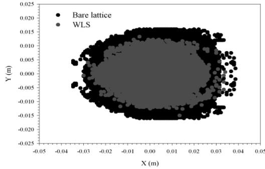
Figure 4. The comparison of the dynamic aperture of bare lattice and the perturbed by wavelength shifter after the tune correction to the bare lattice.
