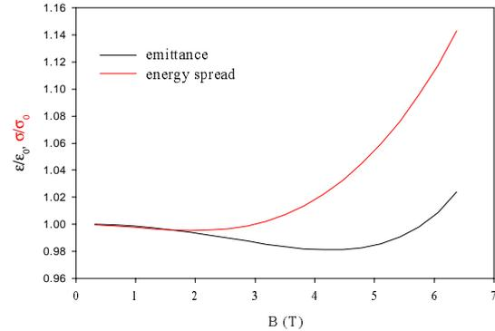
Figure 5. The emittance and energy spread ratio verse the excited magnet field strength of the SWS's on the storage ring.
