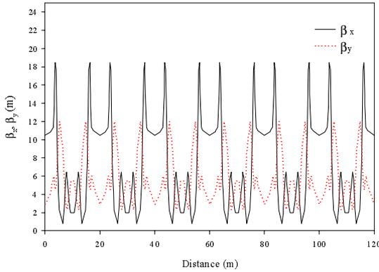
Figure 2: The optics,  $\beta_x$  and  $\beta_y$  of TBA bare lattice
