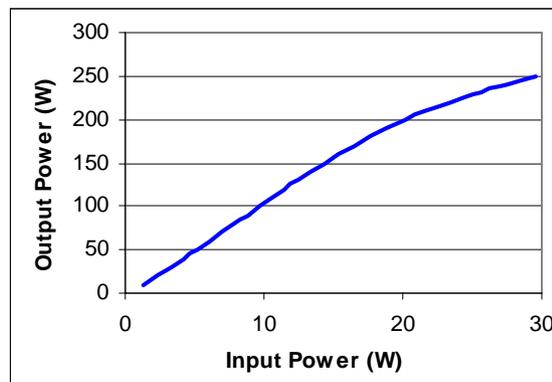
Figure 4: Prototype amplifier module gain curve @ 476 MHz.
