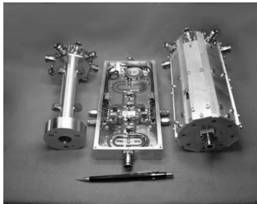
Figure 3: Prototype solid state amplifier module and power combiner/dividers. This module produced 250 W @ 476 MHz.
