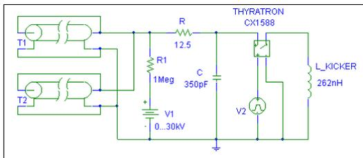
Figure 1: Prototype kicker pulser circuit.
