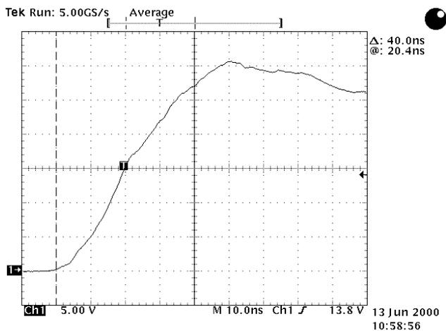
Figure 2 Current waveform in the prototype booster extraction kicker. 20% current overshoot and a 36 ns (5 to 95%) risetime are observed. (65 Amp/div)
