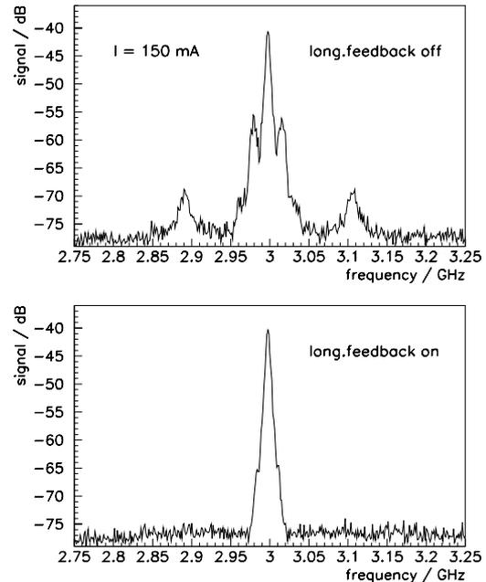
Figure 1: Beam spectrum with LFB switched off (top) and on (bottom), prior to the installation of harmonic cavities.
