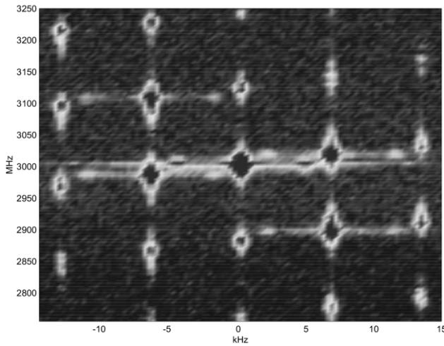
Figure 2: Sequence of spectrum analyzer sweeps of 30 kHz span (horizontal axis) centered at revolution harmonics from 2.75 GHz to 3.25 GHz (vertical axis) prior to the installation of harmonic cavities.
