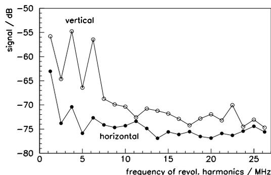
Figure 6: Amplitude of betatron sidebands at 300 mA as a function of the adjacent revolution harmonic frequency.
