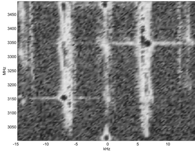
Figure 3: Sequence of spectrum analyzer sweeps of 30 kHz span (horizontal axis) centered at revolution harmonics from 3.00 GHz to 3.50 GHz (vertical axis) after the installation of harmonic cavities.
