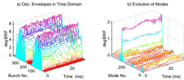
Figure 4: LFB data recorded with zero feedback gain at 390 mA. Shown are oscillation amplitudes versus bunch number (left) and versus mode number (right).
