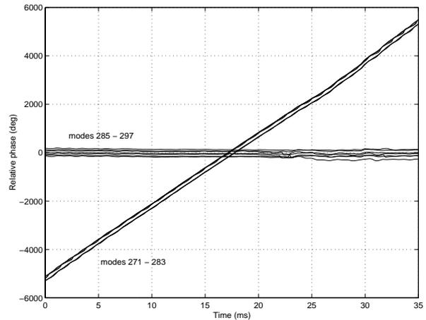
Figure 5: Time evolution of modal phases for multibunch modes selected from figure 4 (plotted relative to the phase of mode 299).
