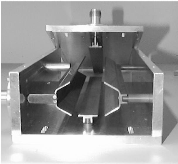
Figure 2: TFB kicker model showing the C-shaped electrodes in horizontal direction and the flat electrodes for the vertical plane
