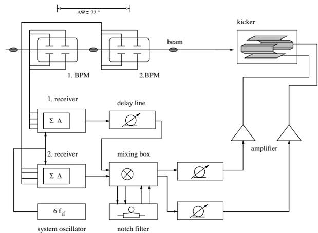
Figure 1: Schematic view of the BESSY II bunch-by-bunch TFB-system
