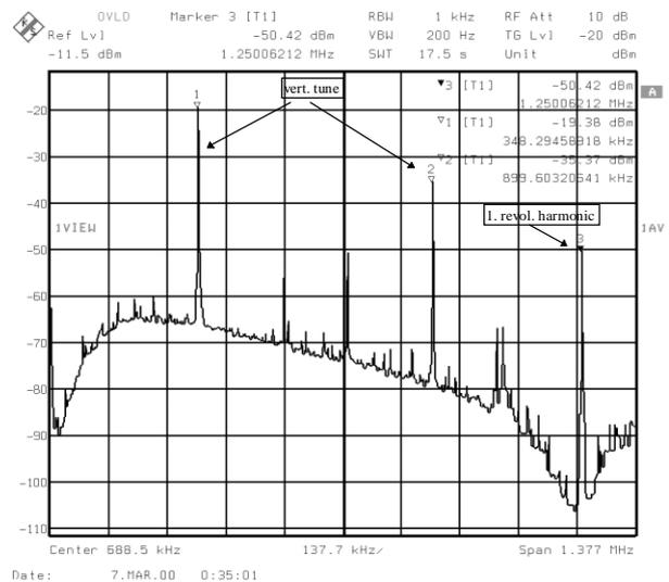
Figure 3: Correction signal in the vertical plane after passing through the notch filter; Frequency range: 0-1.377 MHz
