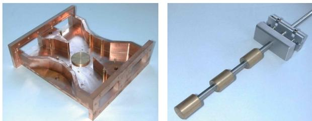
Figure 3 (left): 3 dB coupler layout prior soldering
