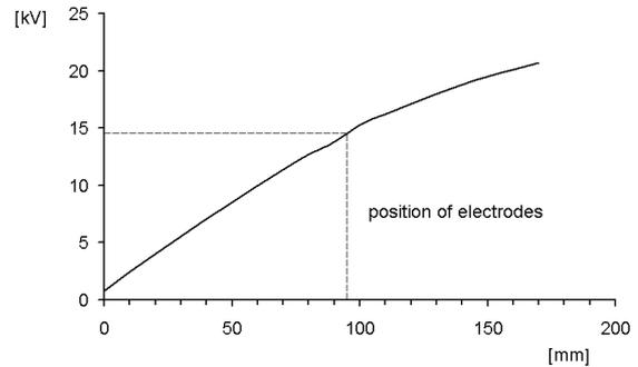
Figure 5: Voltage between the last stem and the tank wall versus stem altitude (RFQ voltage: 70 kV).
