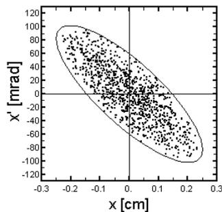
Figure 3: Input particle distribution,  $\epsilon = 150 \pi \text{ mm mrad}$  (same in y-plane).
