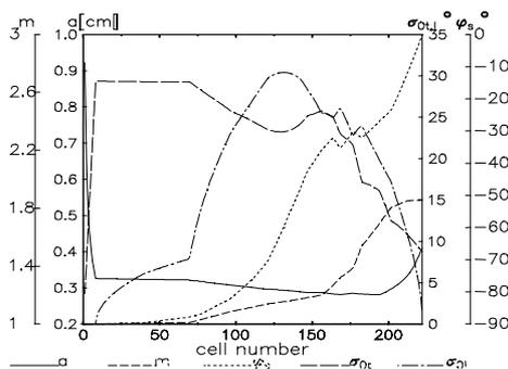
Figure 4: New RFQ design (optimized for bunching with additional drift tubes).
