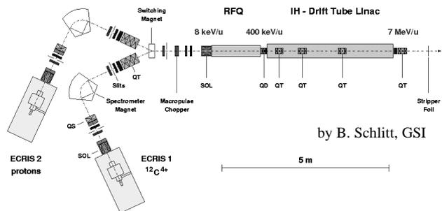
Figure 2: Scheme of the LINAC section.
