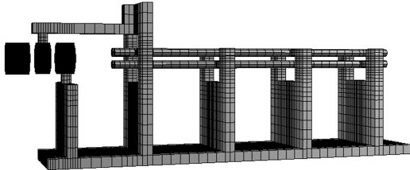
Figure 7: Two bunching gaps (last drift tube is connected to the invisible tank).
