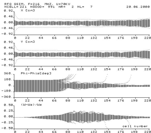
Figure 8: Beam transport within the RFQ electrodes.
