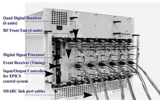
Figure 1: DBPM VME crate for SLS booster commissioning, starting in July 2000. The complete installation includes (from left): one IOC, one timing card, one DSP, 6 RF front ends and 6 QDRs with SHARC link cables.
