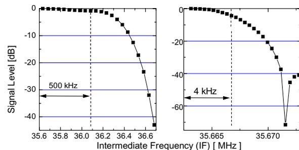
Figure 3: Programmable bandwidth of QDR. (a) 500 kHz for turn-by-turn mode, (b): 4 kHz for closed orbit mode.
