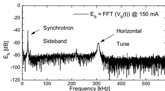
Figure 5: FFT of the turn-by-turn data (see figure 4). Horizontal tune at 300 kHz and synchrotron sideband at 22 kHz can be seen.
