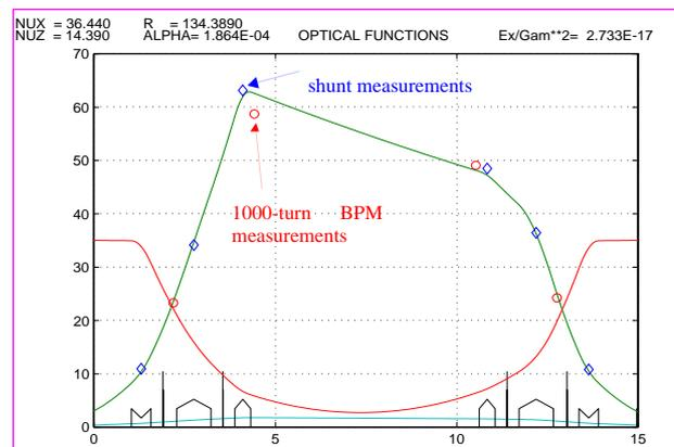
Figure 4: Comparison of measured and predicted  $\beta$ -functions in the HFO straight section
