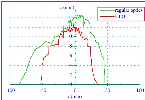
Figure 3: Comparison of the dynamic apertures of the HFO and of the regular optics
