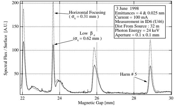
Figure 7: Comparison of spectral flux from one undulator with the HFO and with the regular optics
