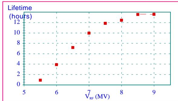
Figure 6: Single bunch lifetime evolution with RF voltage
