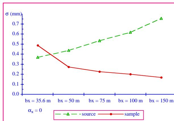
Figure 1: Horizontal rms beam sizes at the source and at the sample for various choices of  $\beta_x$  and  $\alpha_x$
