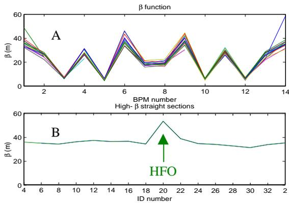
Figure 5: Horizontal  $\beta$ -values along superimposed periods (A) and in the centre of straight sections (B)
