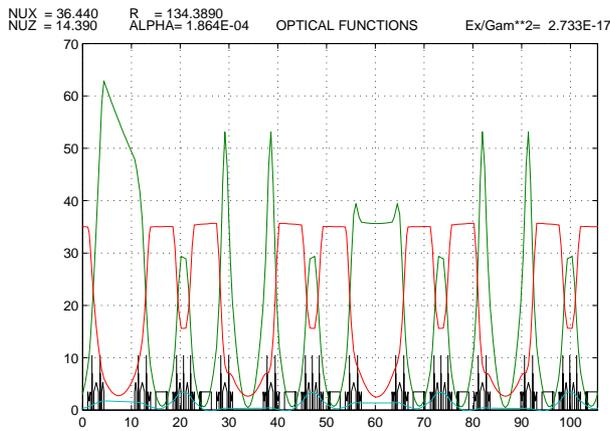
Figure 2: Optical functions for 1 / 8 of the ring
