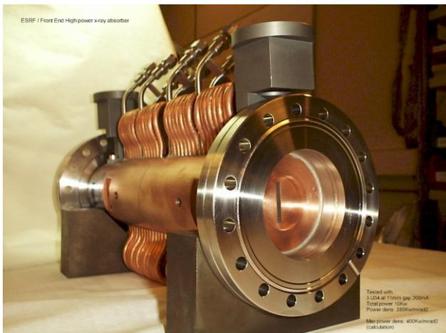
Figure 4: The new high power front-end absorber
