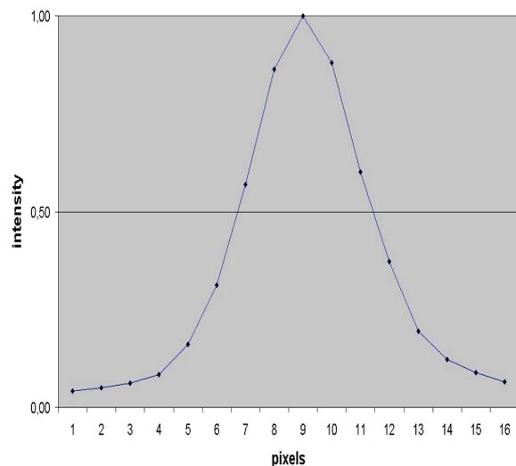
Fig. 2 (b): Cross section of the focused beam
