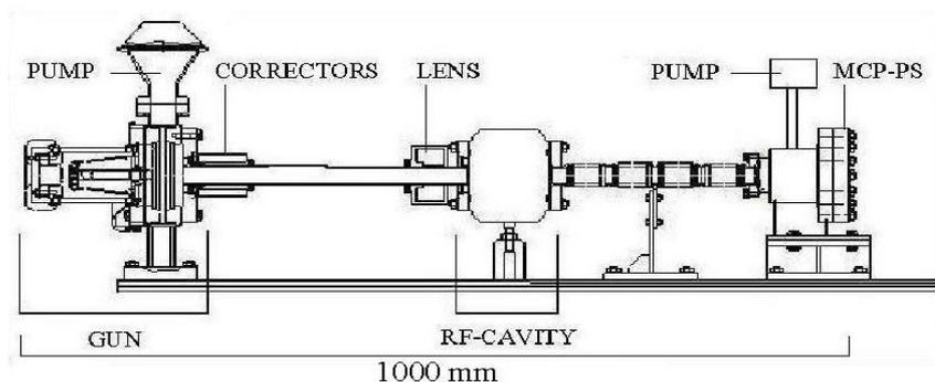
Fig.1: Scheme of the RFC.
