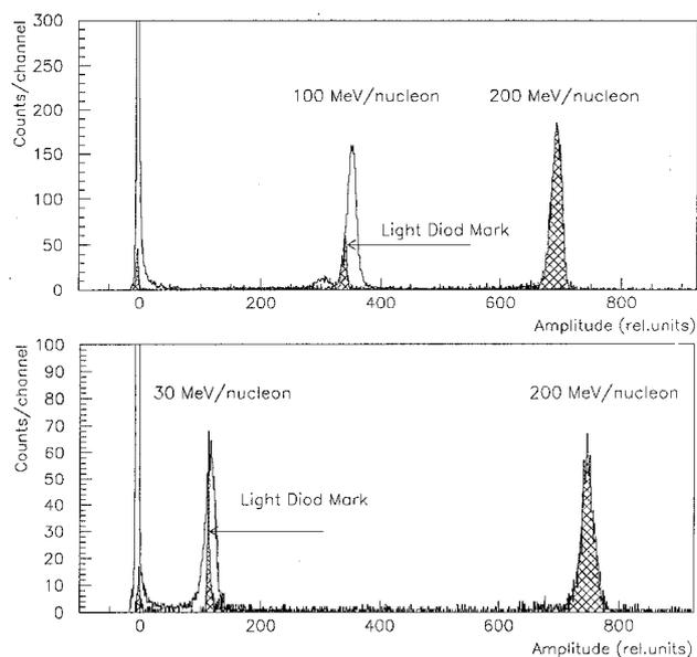
Figure 2: Signals from the beam nuclei and fragments as a number of peaks.
