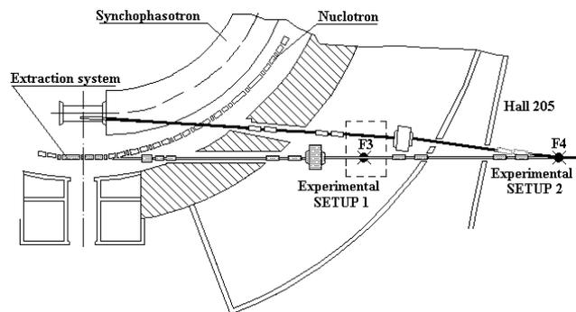
Figure 1: Layout of the beam transport line.
