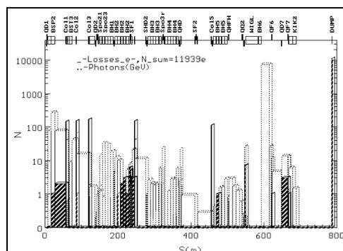
Figure 2: Distribution of leakage particles on an internal surface of collimator.
