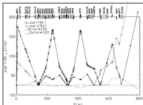
Figure.1: Twiss parameters and dispersion.
