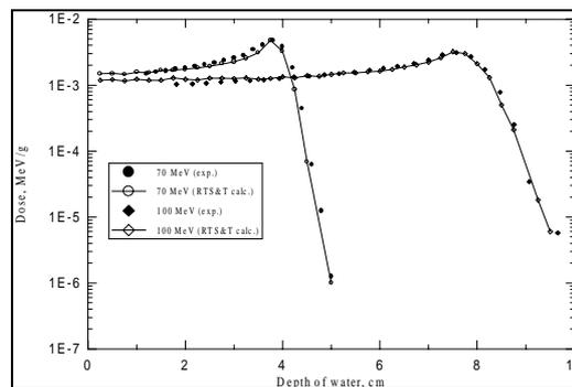
Figure 3: Comparison of doses for 70 and 100 MeV proton beam ( $R_x \times R_y = 30 \times 60$  mm) incident on water slab.
