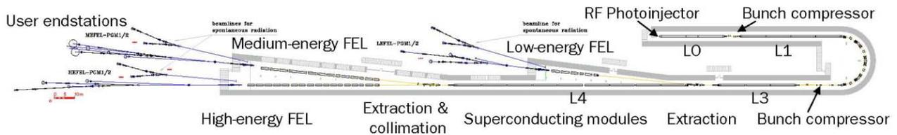
Figure 1: Layout of the main components of the BESSY FEL.
