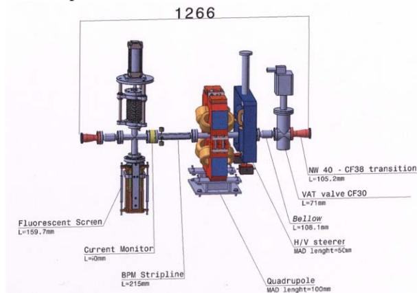
Figure 2: A schematic of intra-sections layout.
