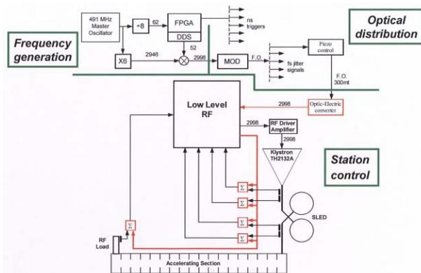
Figure 3: RF Controls system diagram.
