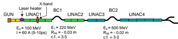
Figure 1: A schematic of the ~150 m long FERMI accelerator.
