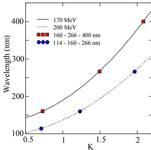
Figure 1: Seeded SPARC FEL operation wavelengths.
