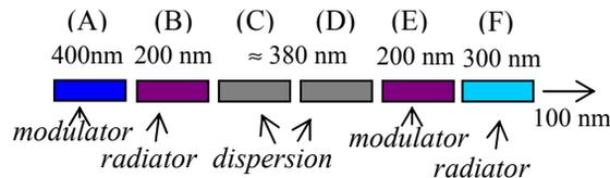
Figure 4: Fresh bunch injection technique layout.
