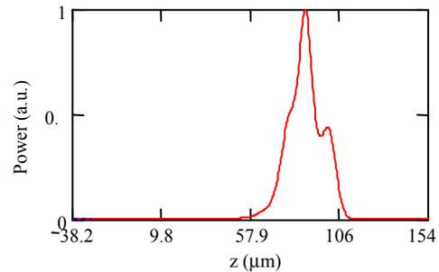
Figure 6: Longitudinal profile of the radiation power at the end of the second undulator.
