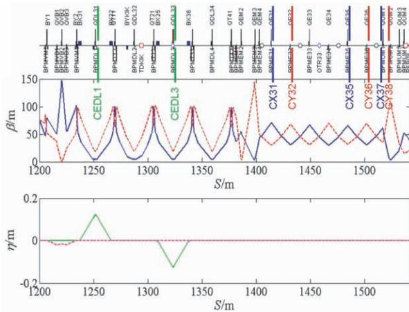
Figure 3: Collimation section in LTU with energy collimators in green,  $x$ -collimators in blue, and  $y$  in red. The undulator starts at the far right side of the plot.
