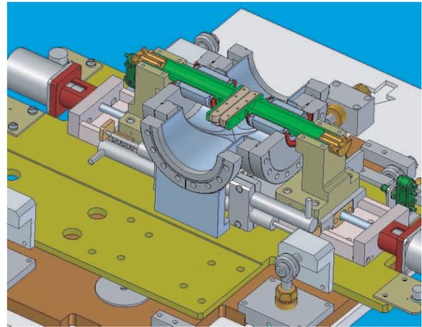
Figure 4: Section view of CE11 with jaws inserted.
