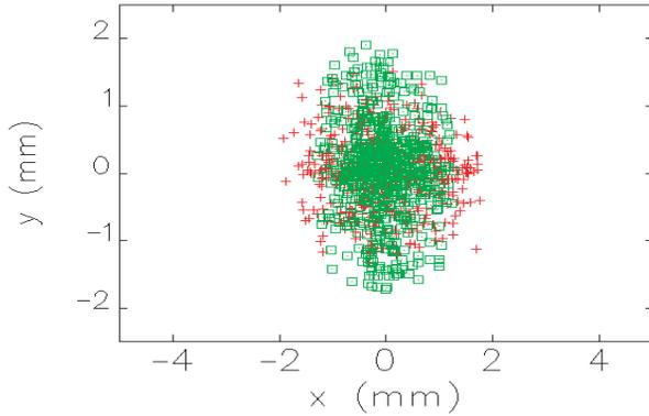
Figure 2: Scatter plot of  $x$  and  $y$  positions of all 614 remaining macro particles/bucket at  $s = 64$  m (red +) and  $s = 43$  m (green square) along the undulator. The plot boundaries represent the vacuum chamber walls.
