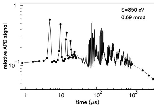
Figure 4: APD signal of 850-eV photons normalized to the short-pulse signal versus time after the laser interaction. Up to 1 ms, a data point is shown for every revolution ( $0.8 \mu\text{s}$ ).
