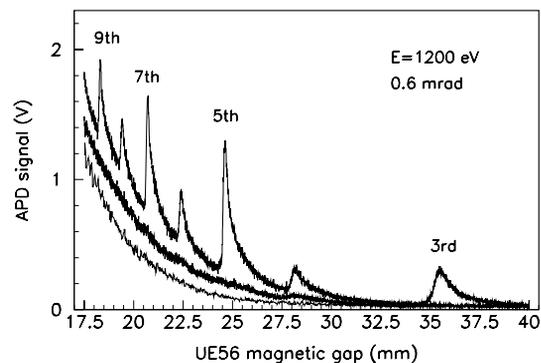
Figure 5: APD signal of 1200-eV photons as a function of the UE56 magnetic gap with and without laser interaction, as well as 1 ms after the interaction.
