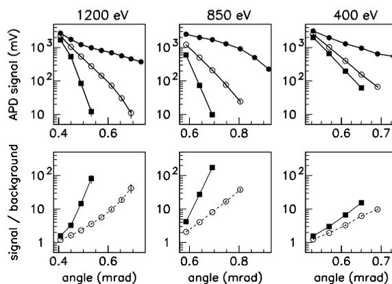
Figure 3: Top – angular distributions of photon signals at 1200 eV, 850 eV and 400 eV with (solid dots) and without laser interaction (squares) and 1 ms after the interaction (open dots). Bottom – ratio of signal and laser-off background (squares) or background after 1 ms (open dots).
