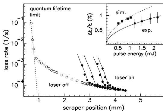
Figure 2: Electron loss rate versus scraper position with (dots) and without (open symbols) energy modulation under variation of the laser pulse energy. The solid lines are simulation results. Inset: modulation amplitude  $\Delta E/E$  versus applied (dots) and simulated (squares) pulse energy. Error bars reflect the uncertainty in the optical functions.
