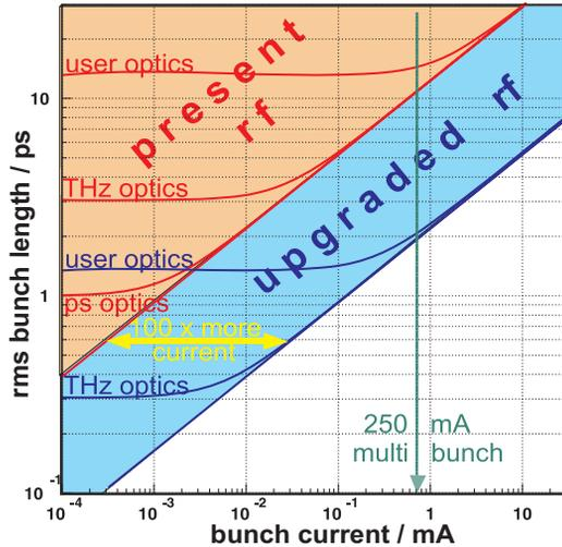
Figure 3: Bunch current relation for the present BESSY II ring (red) and extrapolated version with an 100x upgraded rf-gradient (blue).
