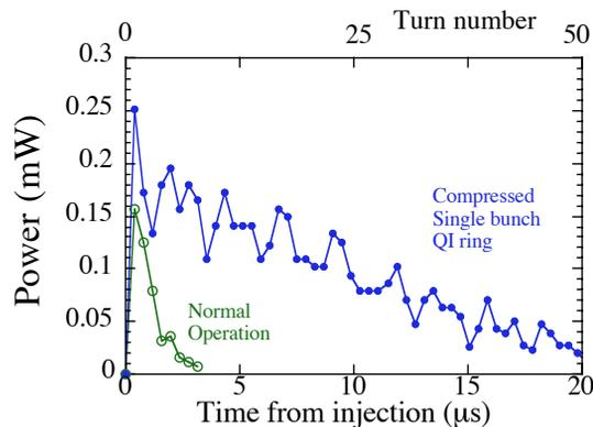
Figure 5: The turn-by-turn CSR power after injection. The line with open circles shows the power obtained with the parameters of normal operation, where there were three bunches in a pulse. The line with filled circles shows the power obtained from one compressed bunch in a QI ring. The bunch charge was about 20 pC/bunch in both cases.
