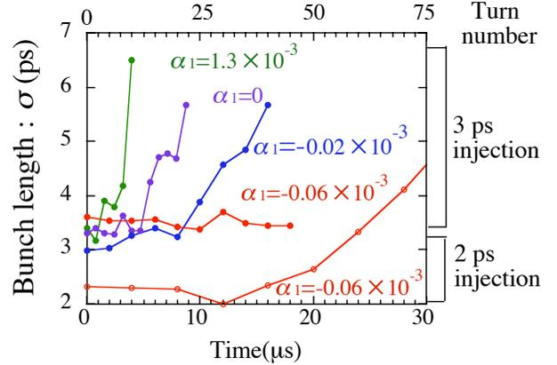
Figure 3: The elongation of the bunch length after injection for different values of  $\alpha_1$ . The initial length was not the shortest, because the buncher phase of the linac was not optimized at that time.
