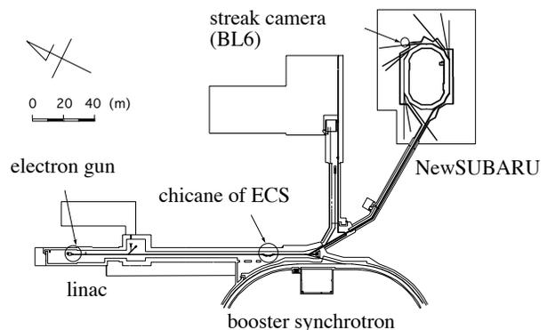
Figure 1: Layout of the SPring-8 linear accelerator, the energy compression system (ECS), the booster synchrotron, and the NewSUBARU storage ring. The streak camera is placed in beamline 6 (BL6) of NewSUBARU.
