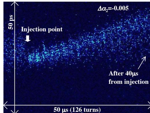
Figure 6: Double-sweep streak camera image with improper  $\alpha_2$ . The vertical axis is the rf phase of the ring and the horizontal axis is the revolution.
