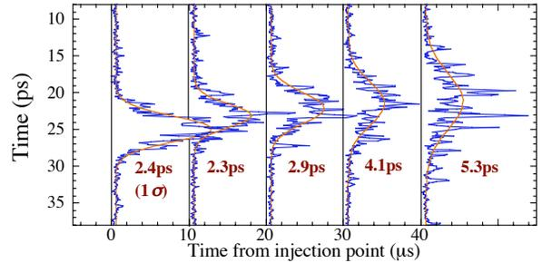
Figure 4: Evolution of the time profile of the bunch after injection, for  $\alpha_1 = -6 \times 10^{-5}$ .
