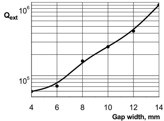
Figure 4: Dependence of  $Q_{ext}$  of a twin coupler on the gap width. HFSS data.
