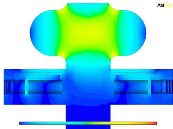
Figure 5: Antenna electric fields distribution.
