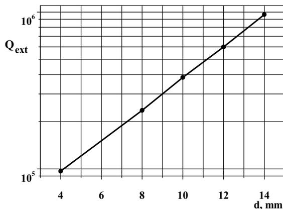
Figure 3: The  $Q_{ext}$  dependence on gap width. ANSYS simulation data.
