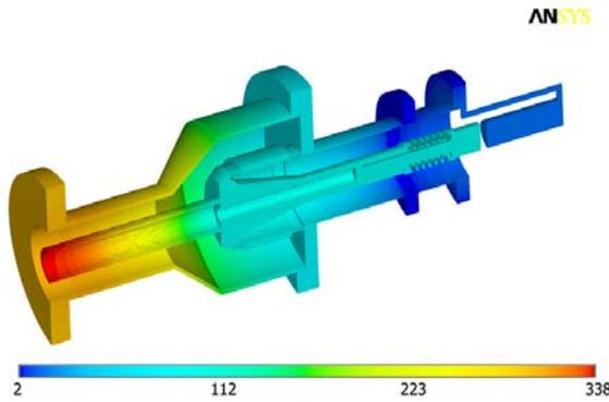
Figure 6: Temperature map of loop-capacitance coupler.
