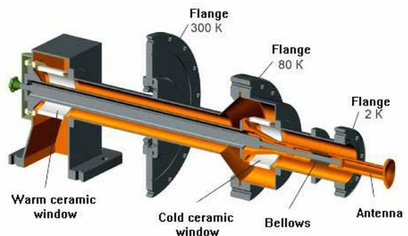
Figure 1: Single bellows coupler.
