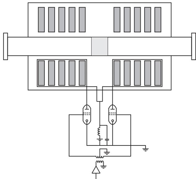
Figure 3: Layout of CR rf cavity circuit.
