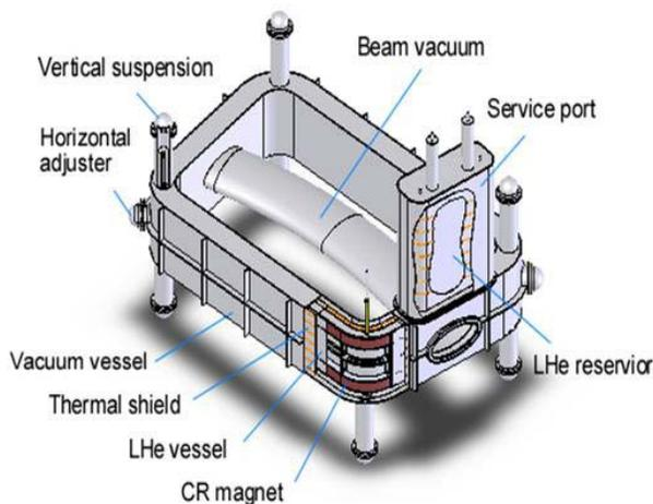
Figure 2: Sketch of CR dipole with cryogenics.
