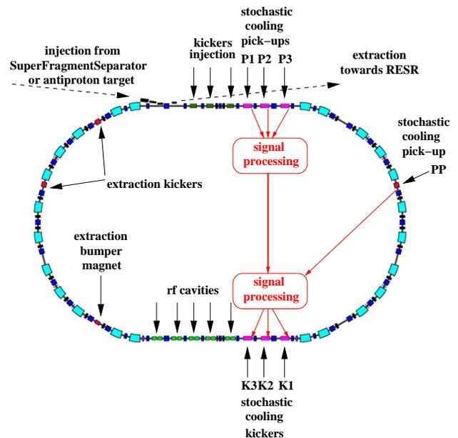
Figure 1: Layout of the CR with stochastic cooling lines.
