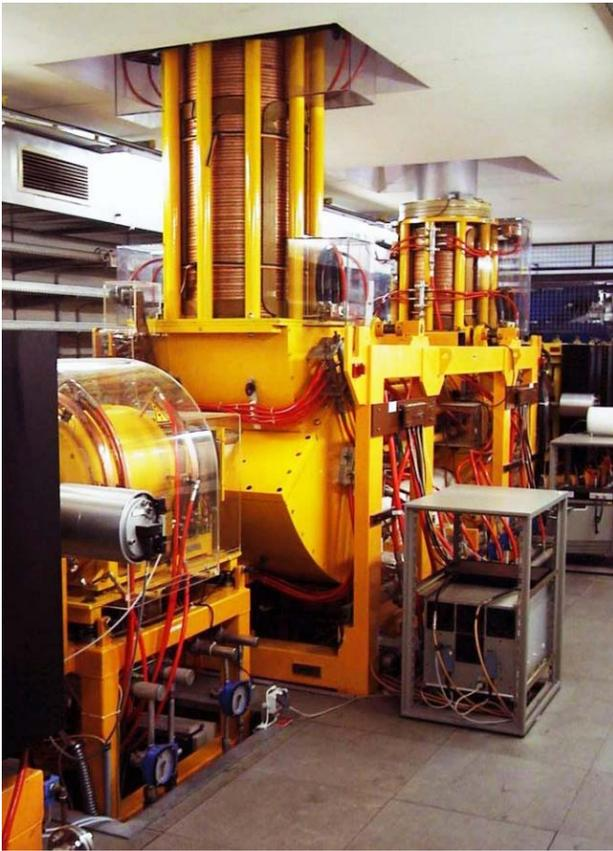
Figure 3: The COSY electron cooler
