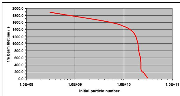
Figure 4: Beam lifetime of 45 MeV protons cooled with a 150 mA electron cooler beam current
