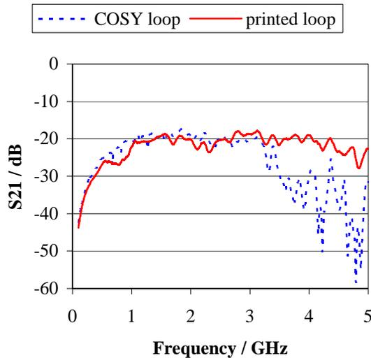
Figure 6: Comparison of COSY-loop and printed loop structures using the test bench of Fig. 5.
