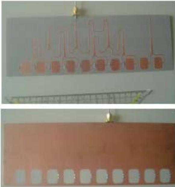
Figure 1: Printed loop couplers (the grid of the ruler is 1cm).
