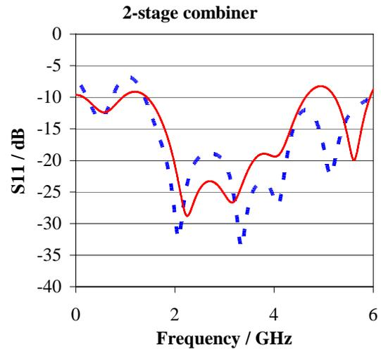
Figure 4: Measured reflection coefficient of one 2-stage combiner including two  $\lambda/4$ -loops (blue) and the corresponding MWS [9] simulation (red).
