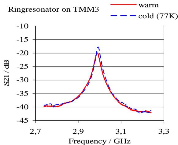
Figure 3: Measured resonance curve of the ring resonator with TMM3 substrate at room temperature and at 77K.
