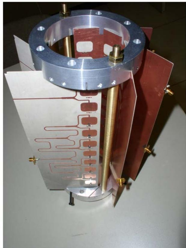
Figure 2: Octagonal pickup structure, equipped with 6  $\lambda/4$ -electrode rows.
