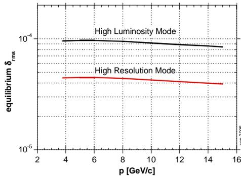
Figure 3: Longitudinal rms equilibrium values versus beam momentum for the HL- and HR-mode.
