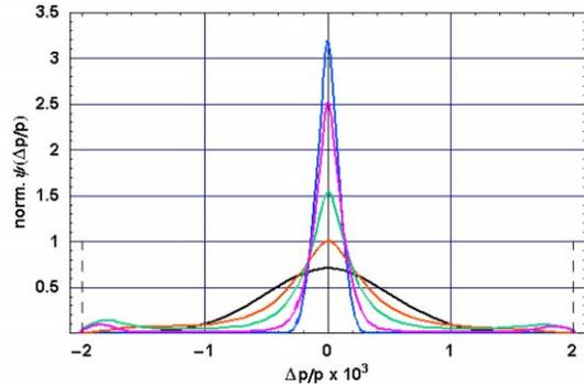
Figure 1: Beam distributions at  $t = 0 s$  (black), 20 s, 50 s, 120 s, 1000 s (blue) for the HL-mode at  $T = 3 GeV$ . The mean energy loss is compensated. The acceptance limit (dashed lines) is set to  $\pm 2 \cdot 10^{-3}$ .
