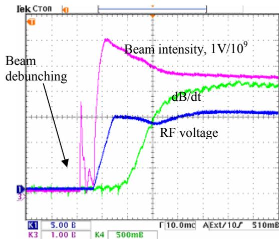
Figure 2: Adiabatic trapping of the beam in booster synchrotron UK.
