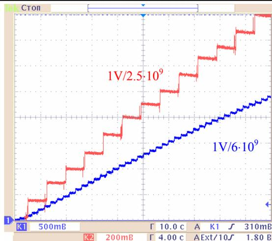
Figure 4: Steps of beam stacking in the U-10 Ring.
