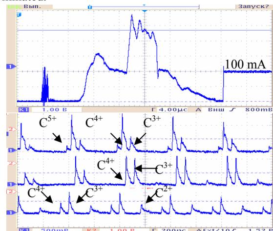
Figure 1: Carbon ions beam at the outlet of the 5J-CO<sub>2</sub> laser ion source.
