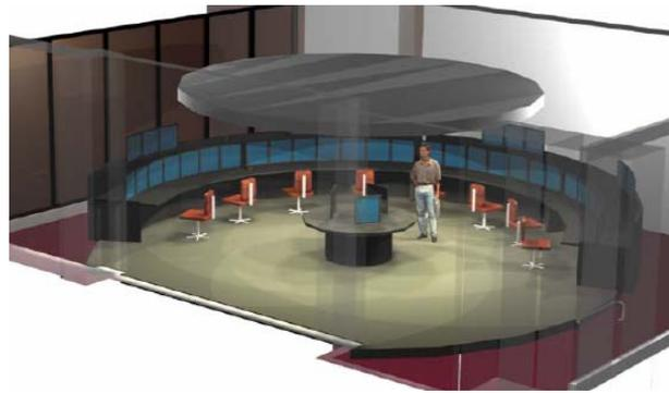
Figure 3, Isometric view of the console layout that can be used for access to personal email and video-conferencing. The entire console configuration encompasses 16 PCs and 40 LCD screens, and can easily be upgraded to double the number of PCs and/or add additional LCD screens.
