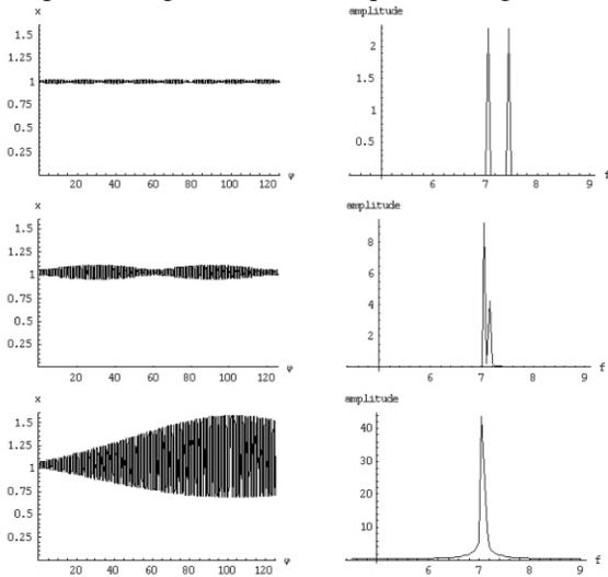
Figure 2: 1D Envelope Oscillations ( $x, \varphi$ ), 20 turns with frequency spectra, approaching resonance. Corresponding parameters are shown in red on Figure 3,  $\Delta Q_e=0.01$ .
