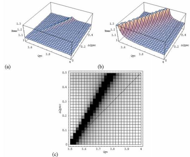
Figure 6: Max. Envelope Amplitudes as a Function of Vertical Set ( $Q_{y0}$ ) and Depressed ( $\Delta Q_{ysc}$ ) Tune, for driven  $2Q_y=7$ . (a) is Horizontal ( $x_{max}$ ), (b) & (c) Vertical ( $y_{max}$ ).
