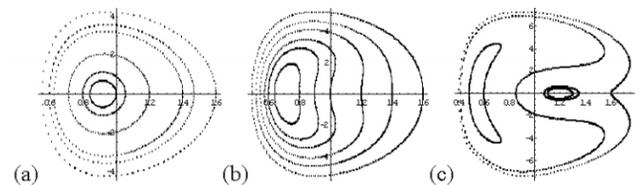
Figure 1: Normalised envelope ( $x, x'$ ) sampled at a given machine azimuth (Poincaré map); (a) above, (b) approaching and (c) “depressed” below resonance.
