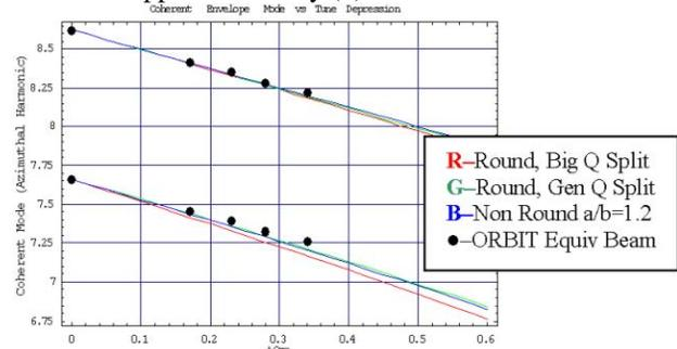
Figure 4: Coherent Frequencies vs  $\Delta Q_{sc}$
