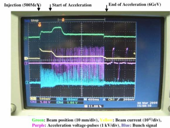
Figure 5: Typical experimental results
