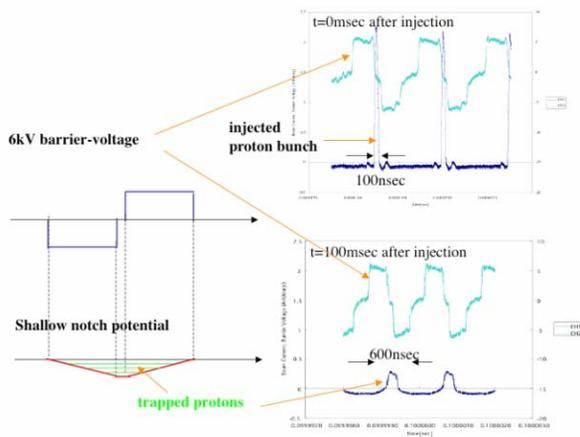
Figure 3: Left, Schematic view of the shallow notch potential; Right, the injected bunch and captured super-bunch with the barrier voltages.
