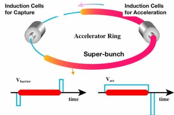
Figure 1: Schematic view of the induction synchrotron.
