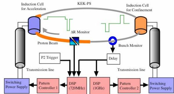
Figure 4: Schematic view of the IS with the gate control system. The induction systems for the acceleration and confinement are of the same type except, for the gate control, which can generate different voltage-patterns, as shown. P2 means the start of acceleration. The signal monitored at the bunch monitor is employed as a master gate trigger signal for the SPSs.
