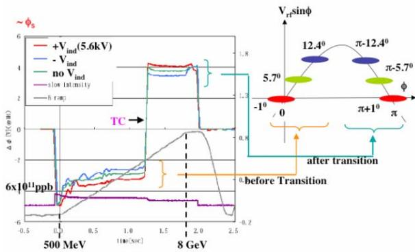
Figure 2: Proof of the induction acceleration of an rf bunch. Left, the phase monitor signals, ramping pattern, and temporal change in the beam intensity; Right, schematic views of the rf bunch and the sinusoidal rf voltage.
