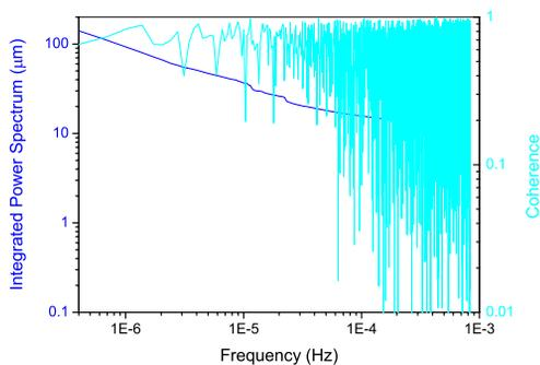
Figure 5: Typical integrated spectrum and coherence between the two positions at a distance of 40m.
