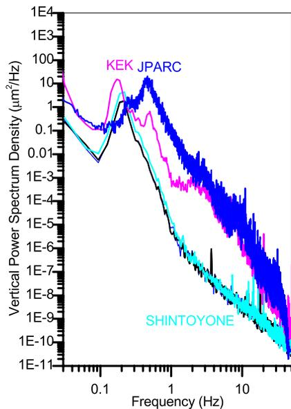
Figure 1: Power spectrum densities obtained on the different geological conditions.
