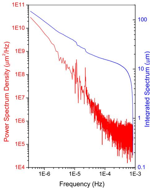
Figure 4: Typical power spectrum density and integrated spectrum obtained by JS-50. Eminent spectrum components around 1E-5Hz regions of frequency are corresponding to the ocean-tide.
