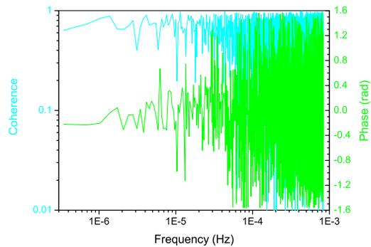
Figure 6: Phase difference and the coherence between the two positions at a distance of 40m.
