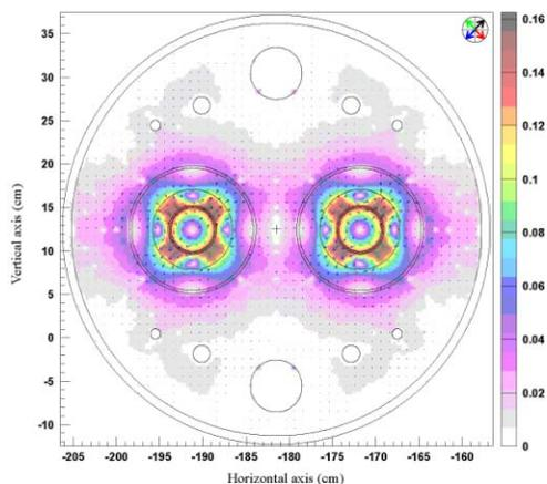
Figure 3: FLUKA field map in T/cm for MQML at 450 GeV.
