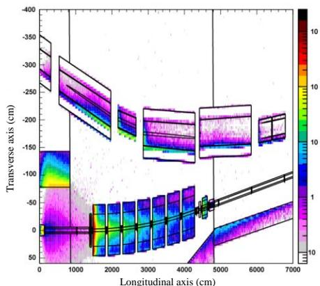
Figure 4: Top view of the simulated geometry after impact on TCDIV.87804. The values are in  $\text{mJ/cm}^3$ .
