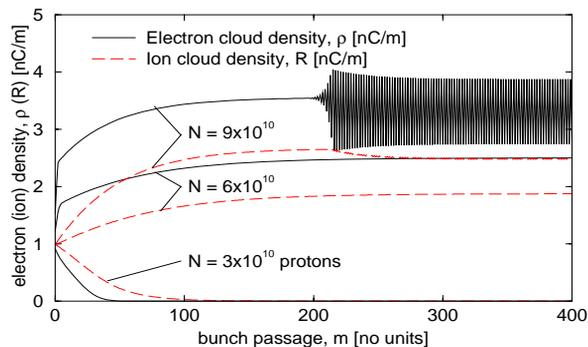
Figure 4: Dynamical evolution of the electron and ion cloud densities as a function of time (bunch passage number) for 3 different bunch intensities,  $N = 3 \times 10^{10}$ ,  $6 \times 10^{10}$ , and  $9 \times 10^{10}$  protons/bunch.
