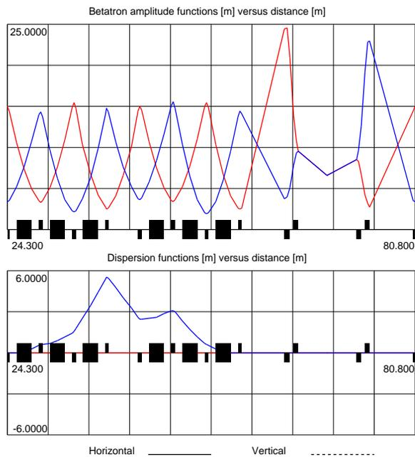
Figure 4: CSNS synchrotron lattice functions.
