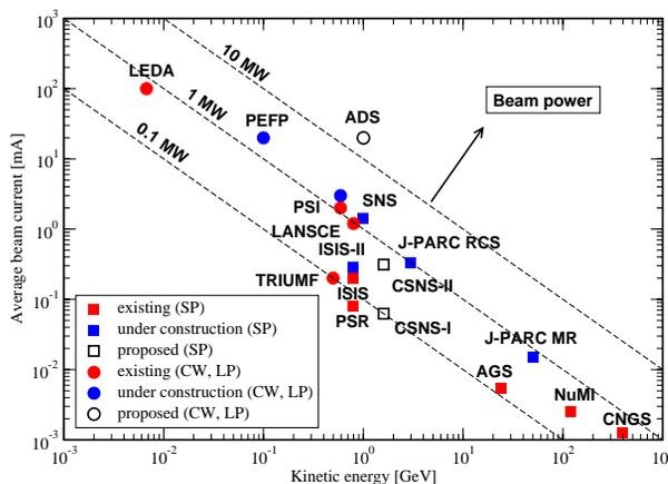
Figure 1: Accelerators at the power frontier (short pulse SP, long pulse LP, continuous wave CW).
