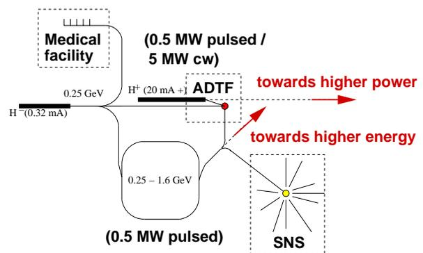
Figure 5: Possible CSNS upgrades towards higher power, higher energy, and multipurpose.
