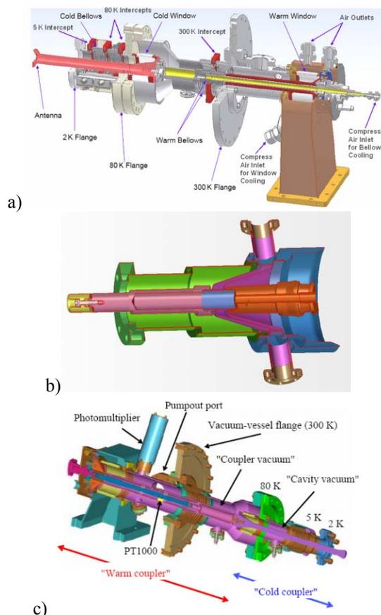
Figure 3: a) Cornell ERL Injector, b) Stanford/Rossendorf and c) TTF III Input Couplers.
