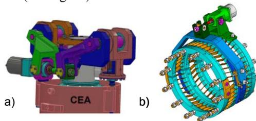
Figure 4: a) Lever-type and b) Blade Tuner Mechanisms.
