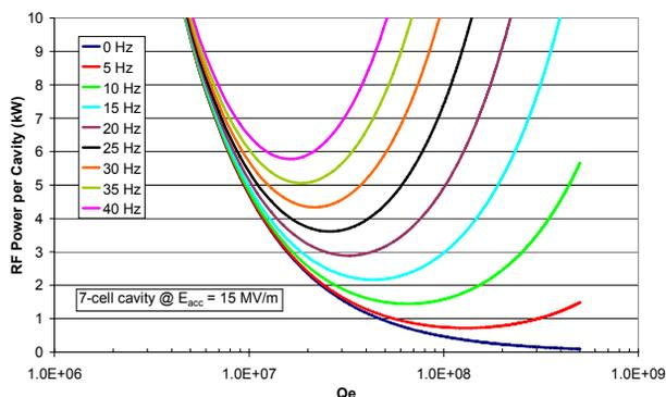
Figure 1: Microphonics Impact on  $Q_e$  and RF Power.
