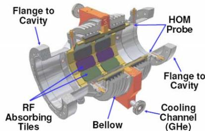
Figure 2: Cornell ERL Injector HOM Absorber.
