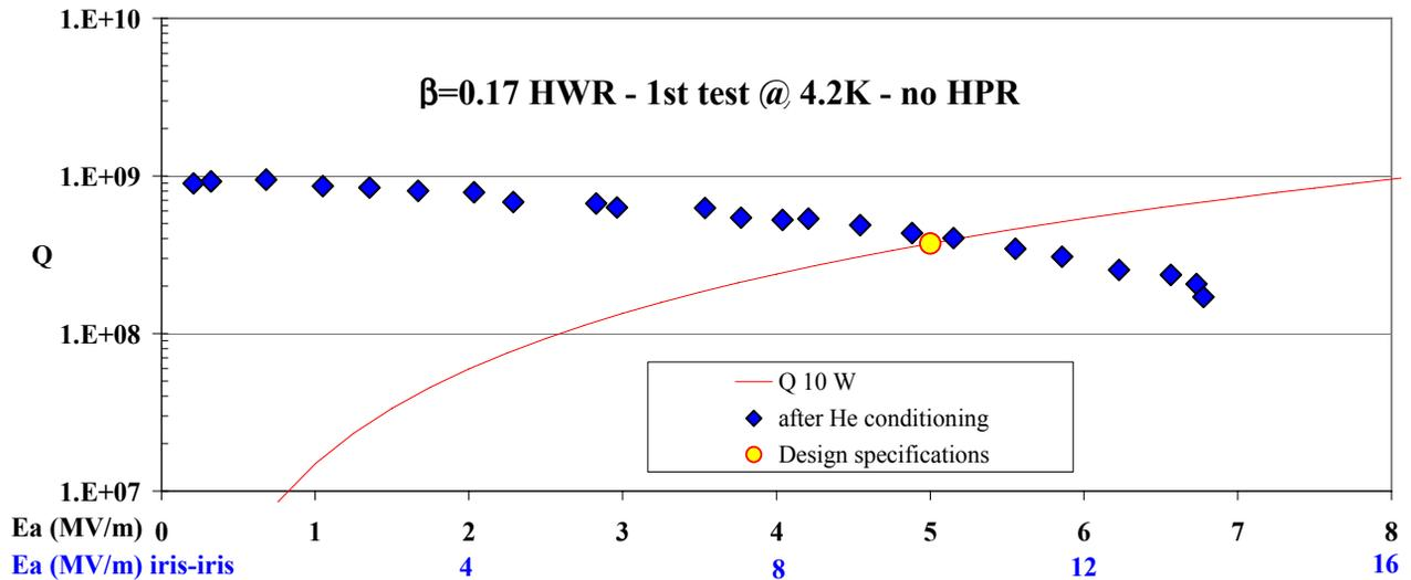
Figure 3: Q vs.  $E_a$  graph at 4.2 K of the  $\beta=0.17$  resonator. The yellow mark represents the design specifications of 5 MV/m at 10 W. Accelerating length: 180 mm = total resonator internal length; to express the accelerating field with the iris-to-iris definition, the  $E_a$  values must be multiplied by 2.
