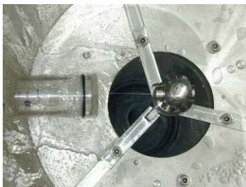
Fig. 1. HPR Test apparatus with luminescence glass plate mounted. Head with six nozzles mounted in the center.
