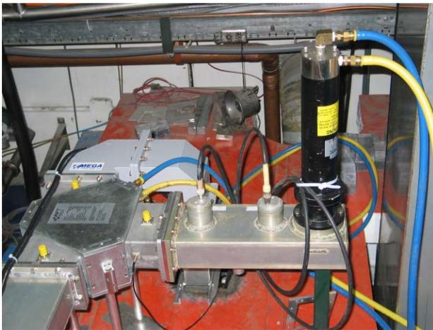
Figure 4: 20 kW CW AFT circulator with RF load.
