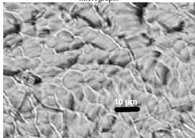
Figure 3c: The PLAD plasma treated sample surface micrograph.
