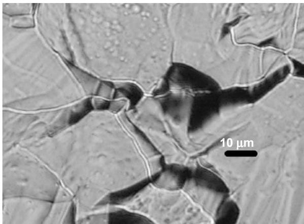
Figure 3d: The BCP treated sample surface micrograph.
