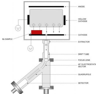
Figure 2: Repetitively pulsed DC diode system [2].
