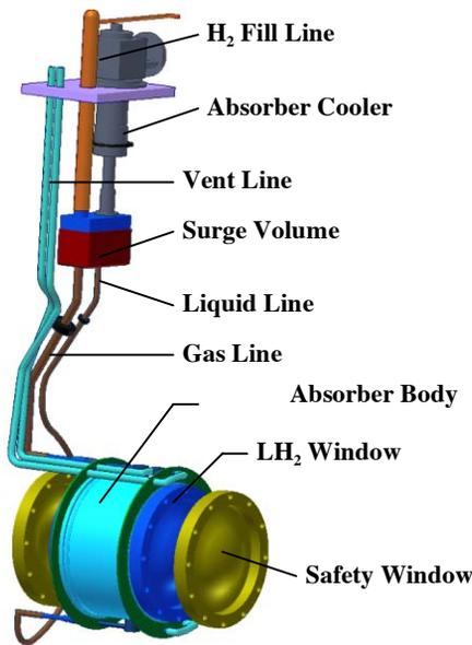
**Figure 1:** 3-dimensional view of the liquid absorber, its cooling system, and hydrogen (helium) supply system.
