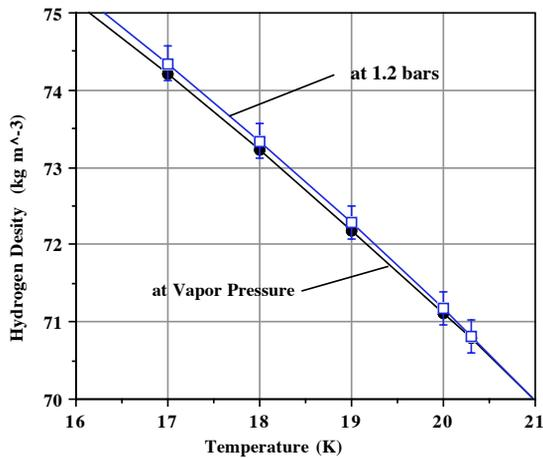
**Figure 4:** The density of liquid hydrogen as a function of temperature at its saturation pressure and at 0.12 MPa.
