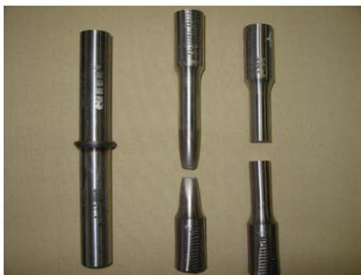
Figure 3: Sample of friction welded Ti-stainless steel joint and the broken samples after a tensile test.
