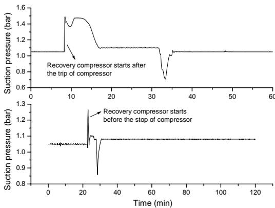
Figure 4: Suction pressure as compressor stops or starts.
