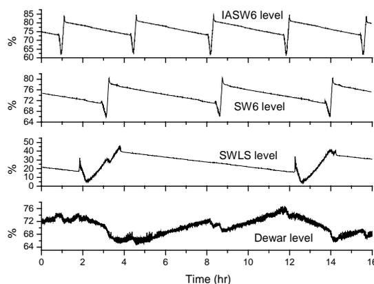
Figure 3: Helium level of magnet cryostats.
