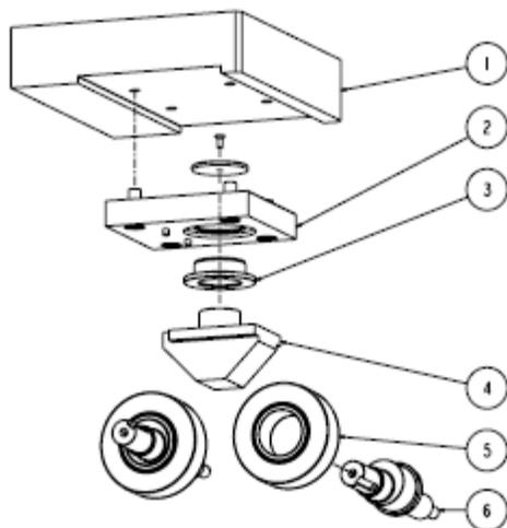
Figure 2: Exploded view of double mover cam.
