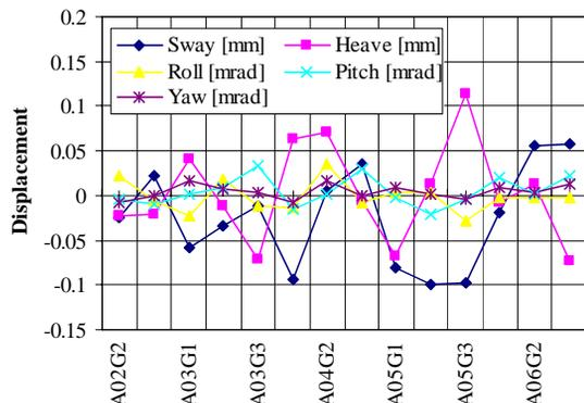
Figure 5: Survey results for selected girders following realignment using remote alignment system.
