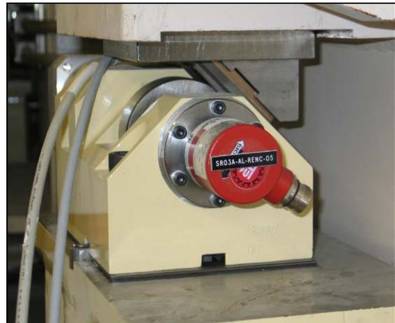
Figure 1: Example cam assembly showing point of contact with girder.
