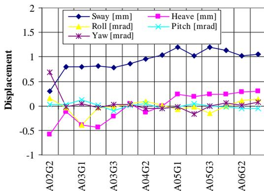
Figure 4: Post-construction survey results. Data shown for girders selected for priority realignment.
