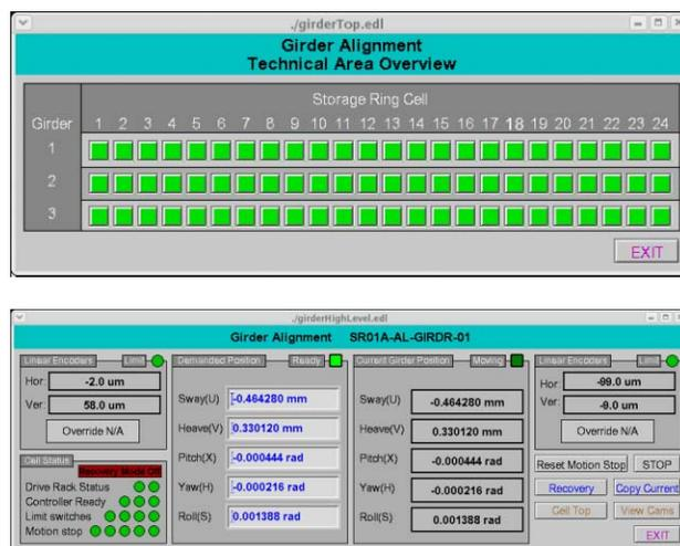
Figure 3: Operator panel indicating ready status for each girder (top) and panel for girder positioning (bottom).
