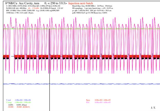
Fig 2a: One revolution in LHC (89 μs) before adaptation: large transients. Red (incident, partly covered by pink reflected trace), pink (reflected) RF power (scale 0-400 kW); green (I), blue (Q) accelerating voltage components (-1 to +3 MV); red bands: bunch energy deviation (scale ±30 MeV); black bands: bunch equilibrium phase (expressed in time, scale ±50 ps). The beam dump gap (close to the left end, no bands) and the kicker-gaps are clearly visible.
