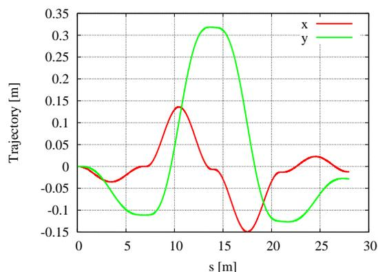
Figure 5: The trajectory inside a 100% helical snake for  $^{241}\text{Pu}^{+94}$  ions at injection ( $\gamma = 10.25$ ) with  $G\gamma = -13.8$ . The offsets at the end of the snake are due to having such large excursions since the field components have a helical sextipole harmonic which increases away from the axis. There is also quite a sizable longitudinal component to the field along the trajectory through the inner two helices (see Fig. 3).
