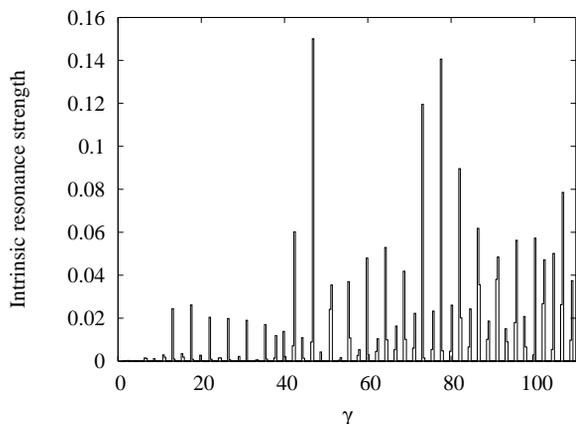
Figure 1: DEPOL calculation of vertical intrinsic resonance strengths for RHIC without snakes. This was for a  $^{241}\text{Pu}$  ion with vertical amplitude corresponding to a normalized 95% emittance of  $10\pi \times 10^{-6}$  m.
