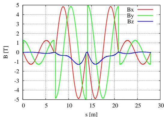
Figure 3: Magnetic field along the trajectory inside 100% helical snake for  $^{241}\text{Pu}^{+94}$  ions at injection ( $\gamma = 10.25$ ) with  $G\gamma = -13.8$ .
