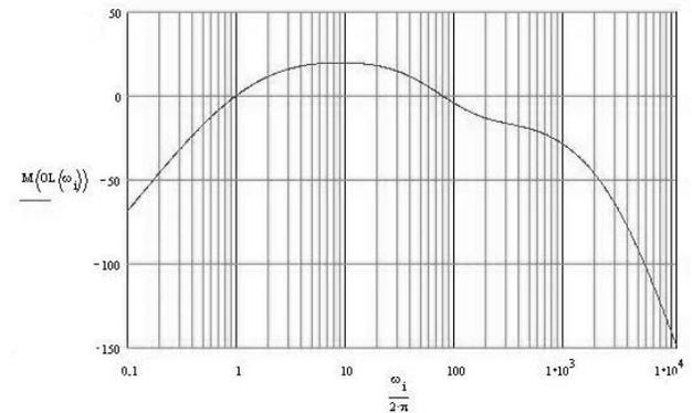
Figure 6: Open loop gain.
