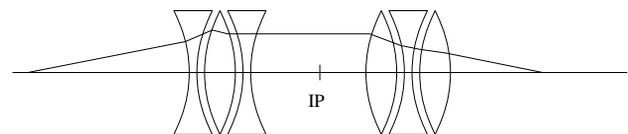
Figure 3: Location of the warm dipole correctors in the focal points of the superconducting low- $\beta$  triplets. Note that the anti-symmetric optics requires different bending angles at the two correctors.
