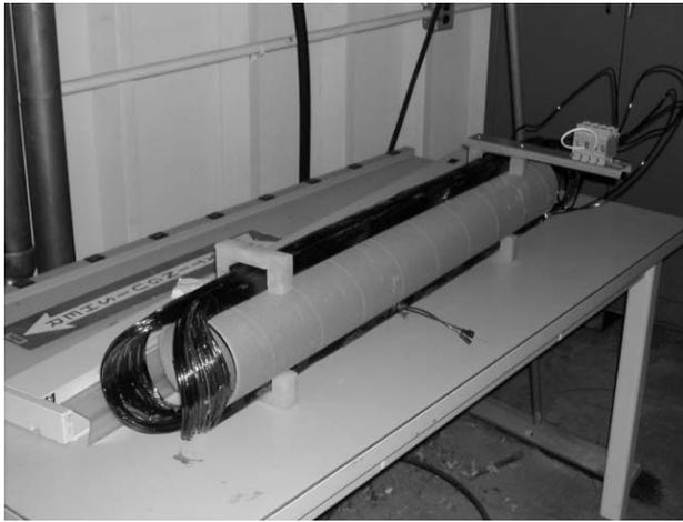
Figure 4: Photo of a correction coil during testing.
