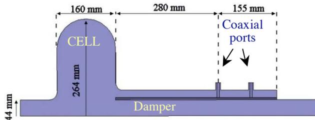
Figure 1: Basic profile of the DAΦNE crab cavity.
