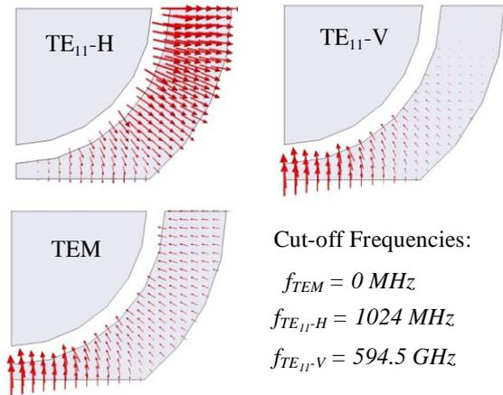
Figure 2: Damper propagation modes - Field distribution.
