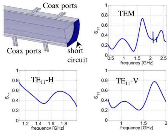
Figure 3: Matching of the damper with coax transducers.
