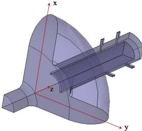
Figure 4: 3D HFSS model of cell and damper assembly.
