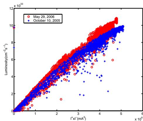
Figure 5: Measured luminosity as a function of product of beam currents for PEP-II. The blue pluses represent the best results achieved in October 2005 and the red circles are data in May 2006.
