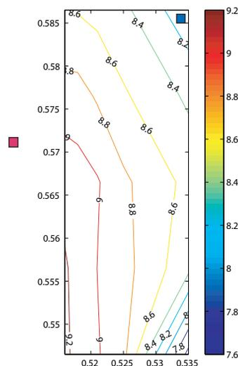
Figure 2: A contour plot of luminosity in unit of  $10^{33} \text{cm}^{-2} \text{s}^{-1}$  in the LER tune plane based on the three-dimensional beam-beam simulation. The blue and red squares indicate respectively the tunes before and after the recent tune change in the LER.
