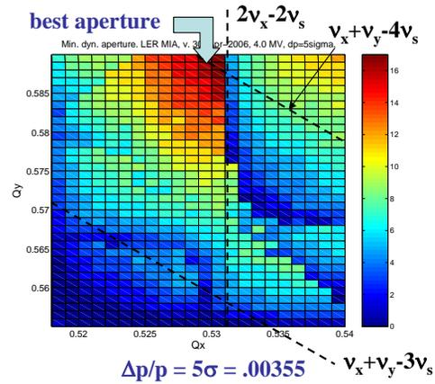
Figure 4: Scan of dynamic aperture in the tune plane using a beam-based model of the LER.
