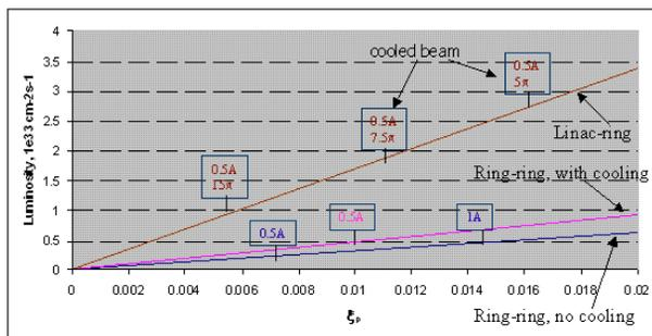
Figure 3: Comparison of the luminosities versus proton beam-beam parameter for the linac-ring and the ring-ring option, with and without the transverse electron cooling of the proton beam. 330 bunches are assumed in the proton ring with  $1 \cdot 10^{11}$  proton per bunch. Markers demonstrate the luminosities for the indicated electron
