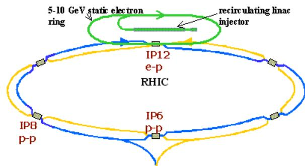
Figure 1: Ring-ring option of the eRHIC uses the electron (or positron) beam from a storage ring for collisions with ions or protons, circulating in RHIC, in one of the RHIC existing interaction points.
