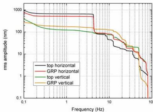
Fig.8: Vessel top to GRP rms amplitude comparison.
