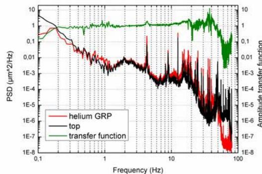
Fig.7: Vessel top to GRP comparison in vertical direction.
