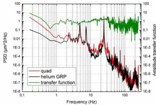
Fig.9: Quad to GRP comparison in transverse direction.
