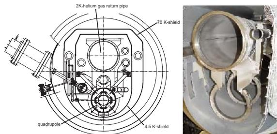
Fig.1: Cross-section of a Type II cryomodule (left) [2], quadrupole support structure (right).
