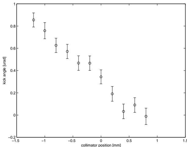
Figure 3: Example of reconstructed angular deflection with collimator 3.
