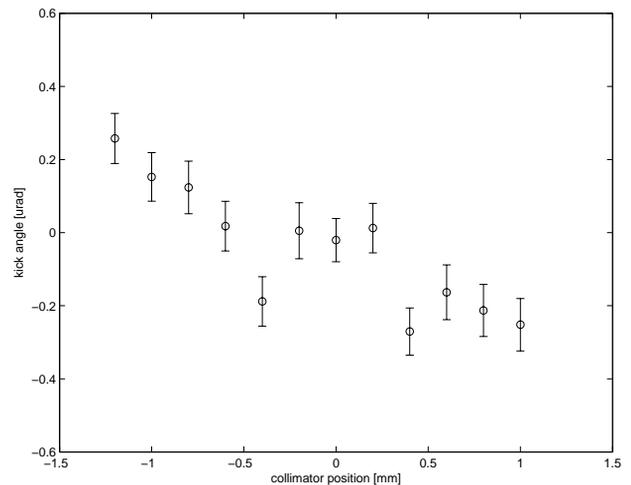
Figure 2: Example of reconstructed angular deflection with collimator 2.
