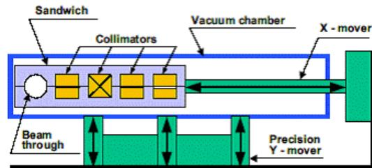
Figure 4: Wakefield Box containing 4 sets of Collimators.
